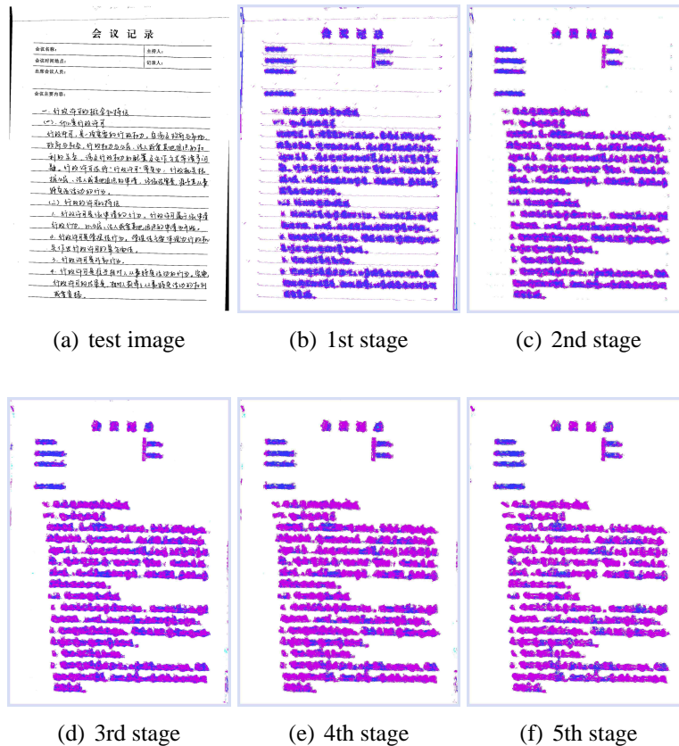
Figure 6.13: A minute page written in Chinese, containing HW and MP contents. At the first stage, HW and MP text regions are located, but their pixels are labeled as mixture of HW or MP. This is difficult, even for human readers, to distinguish one content type from the other. By the fifth stage, most misclassified HW pixels are correct labeled, except for several clusters of characters; most misclassified MP pixels are corrected, except for these lying within the relatively large font title. Note that the pixels on rules are labeled HW in the first stage, and corrected as BL by the fifth stage.
